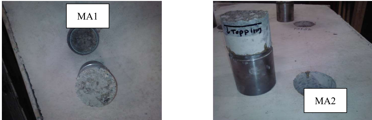
(a) Interface failure
