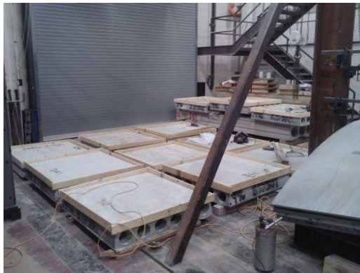
(a) Before casting the topping
