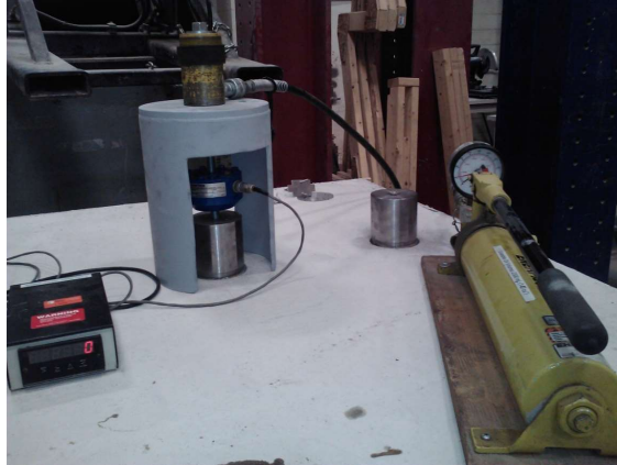
Fig. 6: Pull-off test setup
